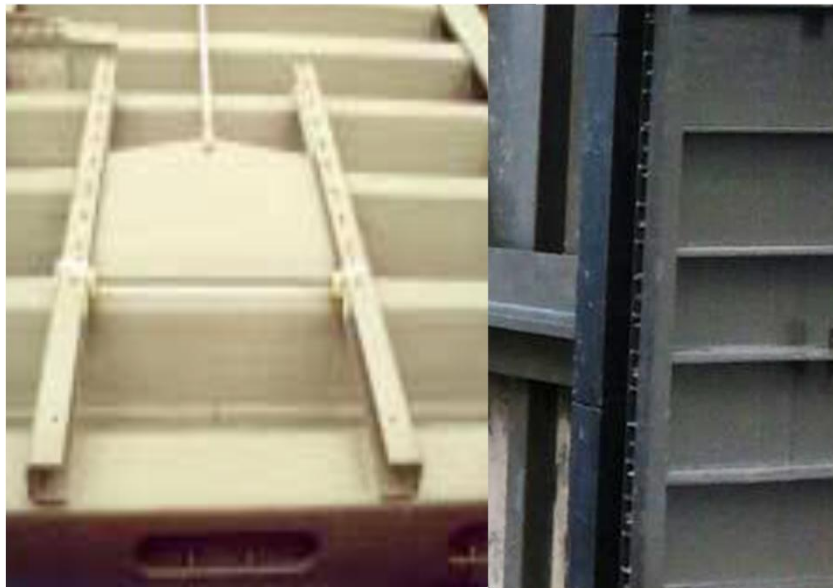
UHMWPE Sliding blocks on Stainless steel
