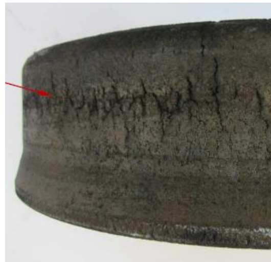
Corrosion fatigue on 12% Mn steel Pivot
